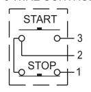
WHEN MORE THAN ONE PUSHBUTTON STATION IS USED OMIT CONNECTOR "A" AND CONNECT PER SKETCH BELOW.
