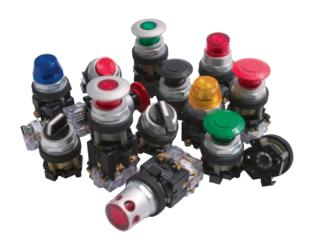
The heavy-duty HT800 Series is a family of 30.5 mm pushbutton devices that includes momentary, illuminated and mushroomhead pushbuttons, selector switches, indicating lights and push-pull units. The HT800 devices have a familiar appearance found in most industrial applications and are suitable for replacement of several other manufacturers' 30.5 mm devices.
