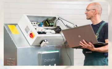
Eaton's XV-102 simplifies servicing - the machine displays the required maintenance and the contact data of the responsible technician.
