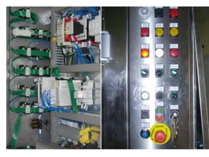
EFC chose a solution including PKZ motor protective circuit breakers, DILM contactors, Easy806 control relay and SmartWire-DT
