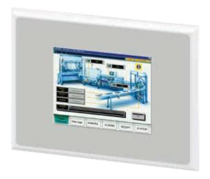
Using the XV-102 touch display, easyE4 users can clearly display the status of their machines and systems and easily adjust parameters.
