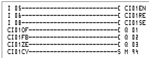
Figure 106: EZD circuit diagram with high-speed incremental encoder counter
