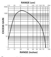
Excess gain is a measurement of how much sensing power a photoelectric sensor has available beyond the power required to detect an object. An excess gain of 1.00 at a given range means there is exactly enough power to detect an object under perfect conditions at that range.
