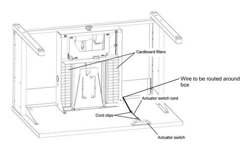
Work surface shown from bottom for ease of illustrating actuator switch installation
