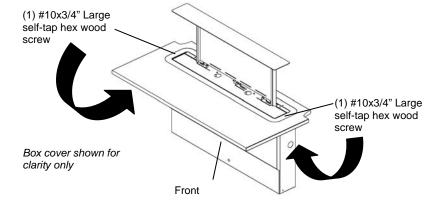
**Note:** At this time, do not install the screws for the rear of the lift frame since it is inaccessible.
