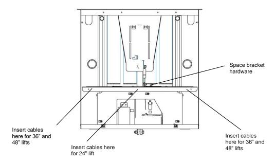
3. Tie together the data cable and AC cable and exit the cable bundle through the monitor hole shown in the following illustration.
