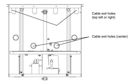
Route the Actuator Switch cord around the box and secure it using the cord clips provided. See the following illustration.
