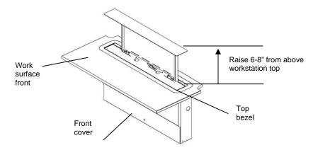
5. With one person on each end of the lift, place your hands inside the top bezel (see figure below), lift the LCD box, and place it inside the work surface opening.
