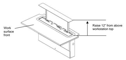
9. If you are installing the lift into a 60" or larger work surface, then ensure the work surface is level before you proceed to the next step.
