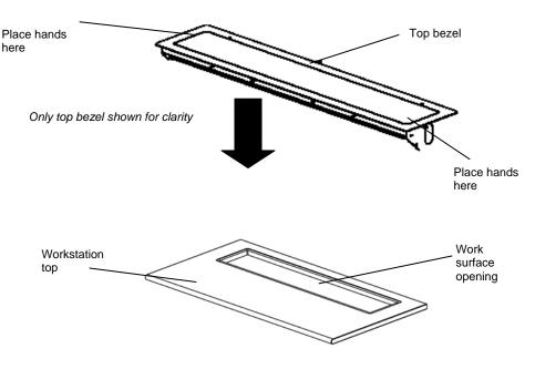
6. Ensure that the lift is properly seated in the desk opening, centered, and flush with the work surface as shown in the following figure.
