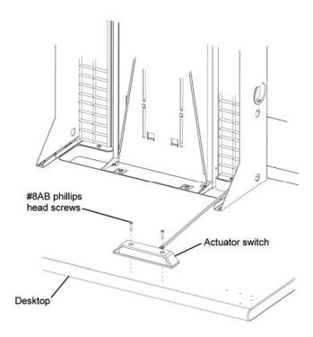
3. Run the Actuator Switch cord either through the center holes or the top left or top right holes shown in the following illustration.
