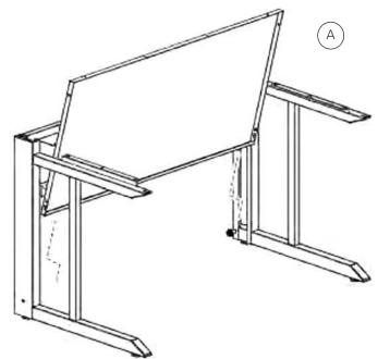
2. Align the slots in the modesty panel with the partially inserted hex screws in both legs. Push the modesty panel in and down to seat the screws in the slots and align the top flange with the bottom flange of the stretcher. The back of the modesty panel must align even with the back of the stretcher.
