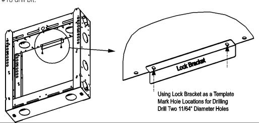
4. Using a #2 Phillips screwdriver, attach the lock bracket to the core with two #10-24 x 3/8" Phillips, pan-head, black oxide, thread forming screws (PN 66714).
