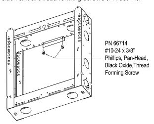
5. Attach removable locking core skin panel to core and lock into place, as shown below.
