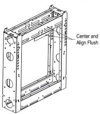
3. Use the lock bracket as a template to mark holes for drilling. Then drill two 11/64" holes using a #18 drill bit.
