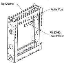
2. Align flange on lock bracket flush with the edge of the top channel assembly, as shown below.
