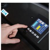
controller shuts down the fans, heater and task light and the display goes into sleep mode. Once motion is detected, the unit powers up the fans, heater and task lights to the last known settings
