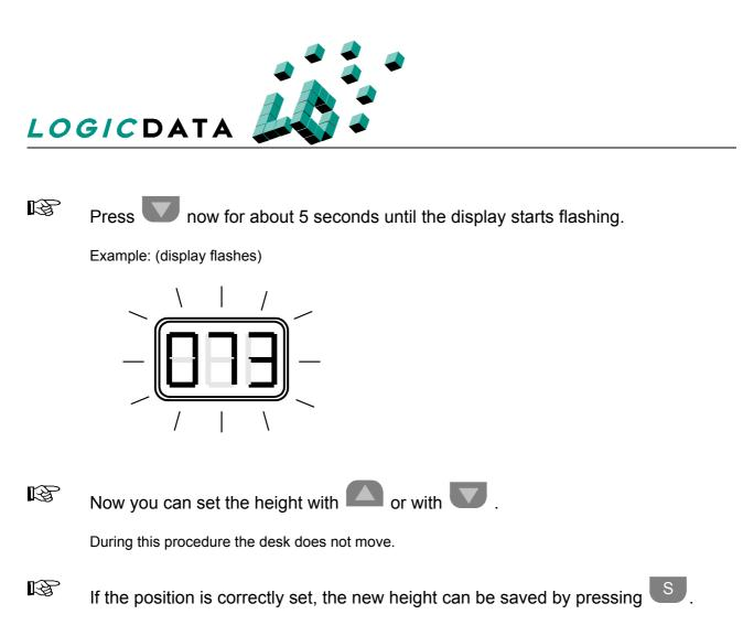
The position is saved and the display stops flashing.
