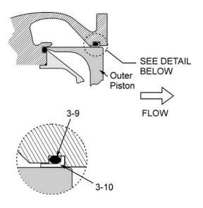
Outer Piston Seal Installation FIGURE 6
