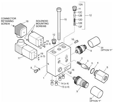
Figure 2 - MANIFOLD PARTS BREAKDOWN
