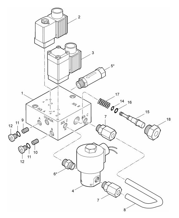
Figure 1 64304 Digital Manifold
