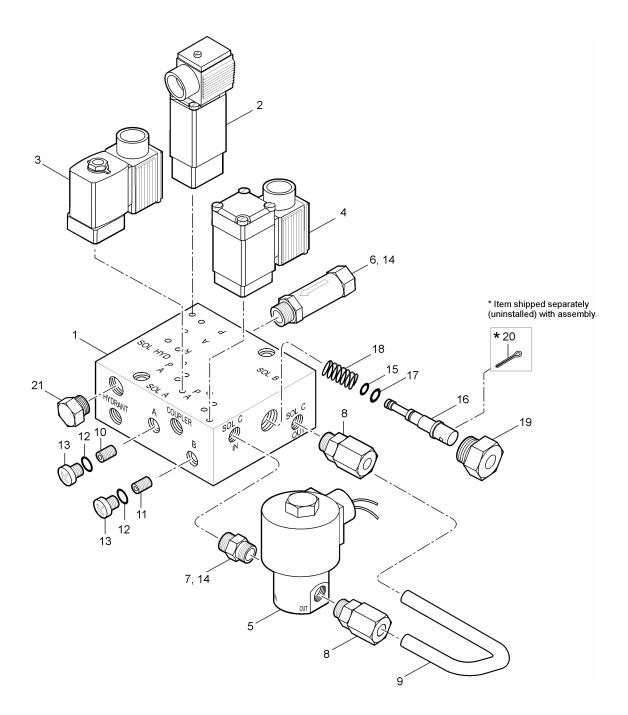
Figure 1 64303 Digital Manifold
