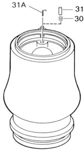
Fig. 3A Continuity Clip (31A) Installation
