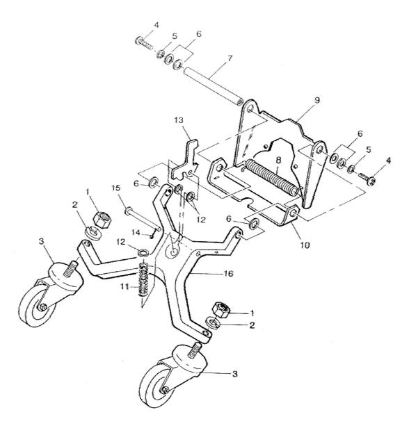
FIGURE 8 60532C CARRIAGE ASSEMBLY OPTION W TO 64902
