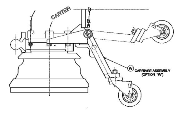
The carriage is assembled by removing four (4) of the Nuts (3-3) and Washers (3-2), placing the carriage in place and reinstalling the nuts and washers as noted in paragraph 11.9.D.
