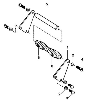
FIGURE 13 STANDARD TRANSVERSE CARRYING HANDLE
