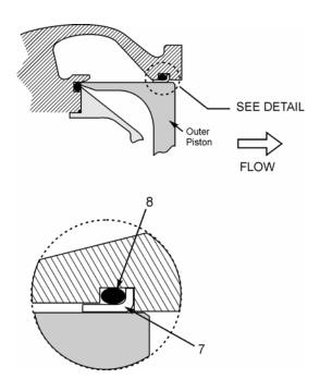
FIGURE 12 OUTER PISTON SEAL INSTALLATION
