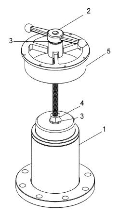
Figure 5 Spring Compression Tool- TF64191-2
