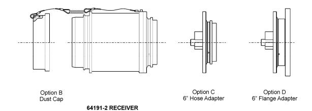
Figure 1 7" Emergency Breakaway Probe & Receiver with Options
