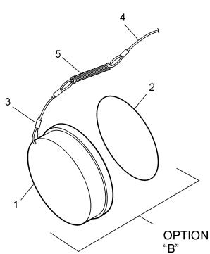
Figure 3 7" Emergency Breakaway Receiver- Protection Cap Female Option B
