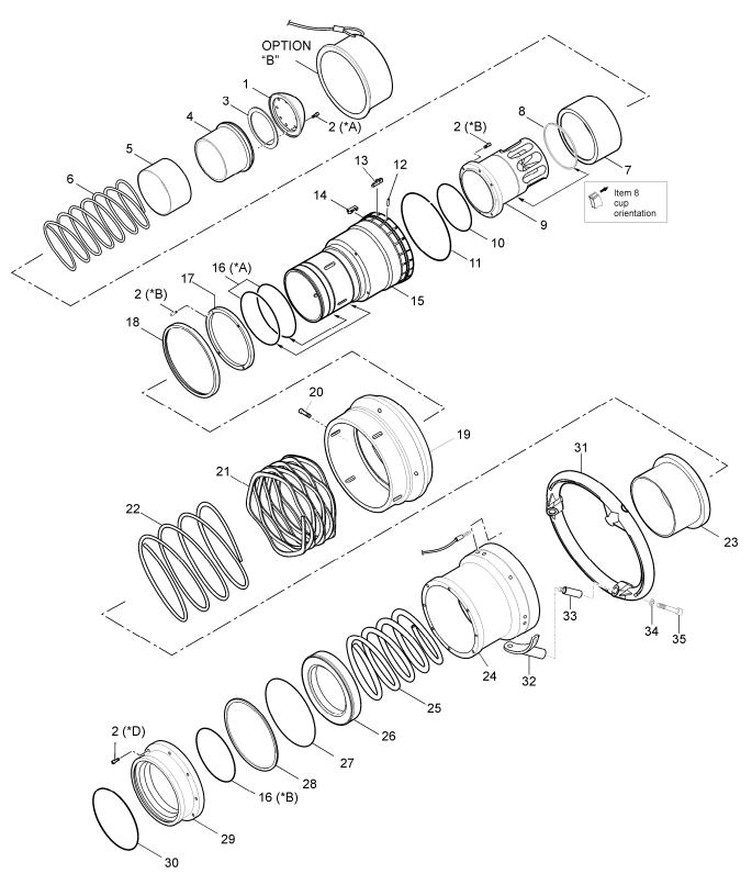
Figure 2A 64191-1 7" Emergency Breakaway Probe (Probe)
