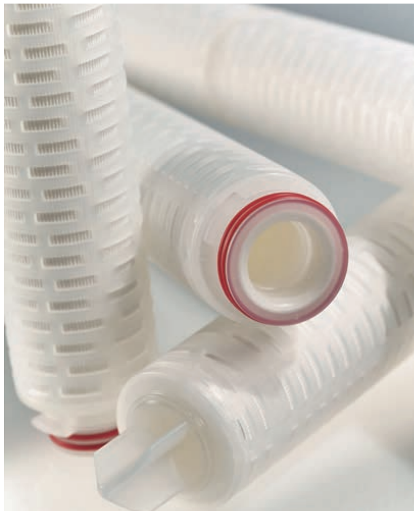
Beco membran PFplus and PS are pleated membrane filter cartridges made of polyvinylidene fluoride (PVDF) or polyethersulfone (PES) that can be tested for integrity.
