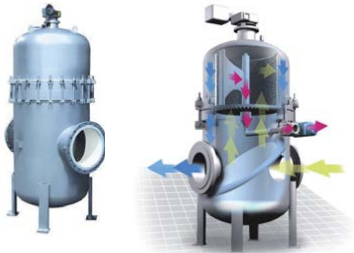
Eaton Model 2596 automatic self-cleaning strainer has flow rates of up to 35,000 GPM (7,950 m 3 /h), a broad selection of screen options, automatic backwashing and exclusive idL seal for leak free service, this strainer is designed for continuous, uninterrupted removal of entrained solids from liquids in pipeline systems.
