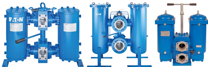
Duplex filter configurations can operate continuously. When a filter element changeout or service is required, filtration flow can be diverted from one side to the other. A pressure equalization system will ensure consistent pressure while the flow is being transferred.
