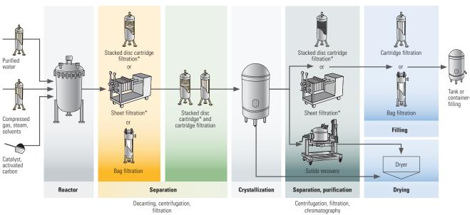
\* Eaton depth filter sheets meet national and international quality standards, such as Regulation (EU) 1935/2004 and FDA guidelines (Food and Drug Administration) from the USA. The plastic components of the stacked disc cartridges (polypropylene) meet Regulation (EU) 10/2011.
