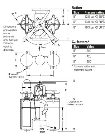
Partial cutaway of Model 50 duplex strainer clearly illustrates all major parts-and gives a clear indication of the simplicity of design and ease of maintenance.
