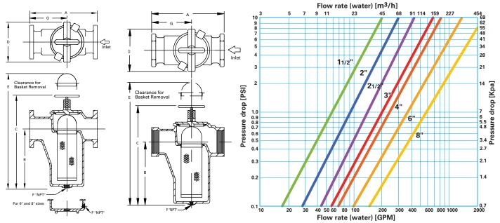
Dimensions and weights are for reference only. Contact Eaton for certified drawings.
