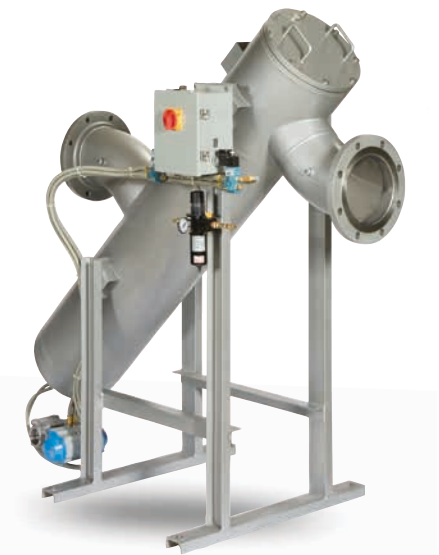
MCS-1500 strainer is perfect for high-capacity needs. Its magnetically coupled actuation eliminates the need for dynamic seals.
