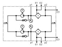
Filter unit with electrical clogging indicator AE30
