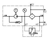
Filter unit with visual clogging indicator AOR, AOC, OP
