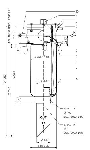
2) Connection for the potential equalization, only for application in the explosive area.
