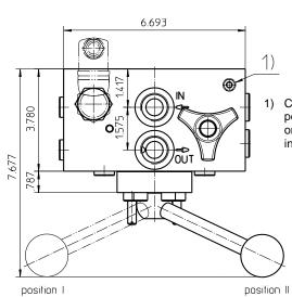
Connection for the potential equalization, only for application in the explosive area.
