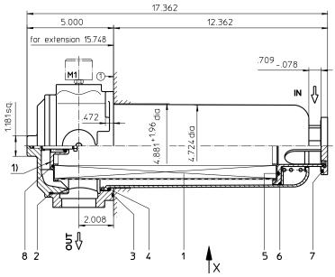
1) The bypass valve is integrated in the screw plug. For the filter without a bypass valve the opening function is raised up to  $\Delta p > 14.5$  PSI.
