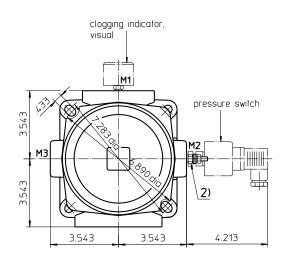
2) Connection for the potential equalization, only for application in the explosive area.
