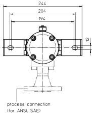
1) Connection for the potential equalization, only for application in the explosive area.
