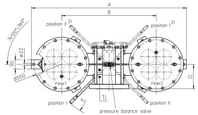
1) Connection for the potential equalization, only for application in the explosive area.
