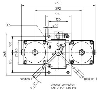
Connection for the potential equalization, only for application in the explosive area.
