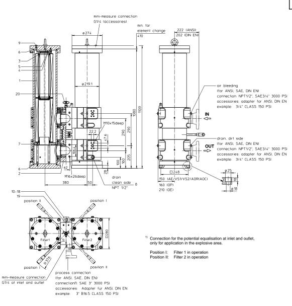
STAINLESS STEEL-PRESSURE FILTER, change-over Series EDA 2214 NPS 3" CLASS 150 PSI
