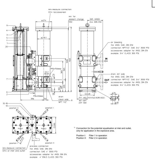
STAINLESS STEEL-PRESSURE FILTER, change-over Series EDA 2205 NPS 4" CLASS 300 PSI Sheet No. **2178 C**
