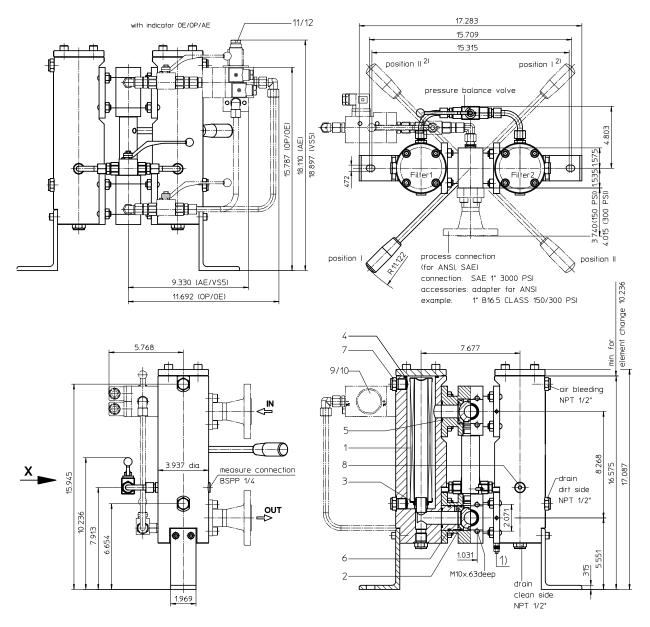
Position I: Filter 1 in operation Position II: Filter 2 in operation
