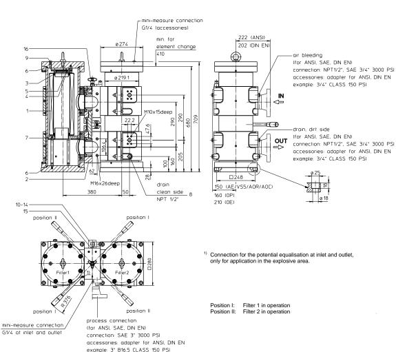
STAINLESS STEEL-PRESSURE FILTER, change-over NPS 3" CLASS 150 PSI Series EDA 1014
