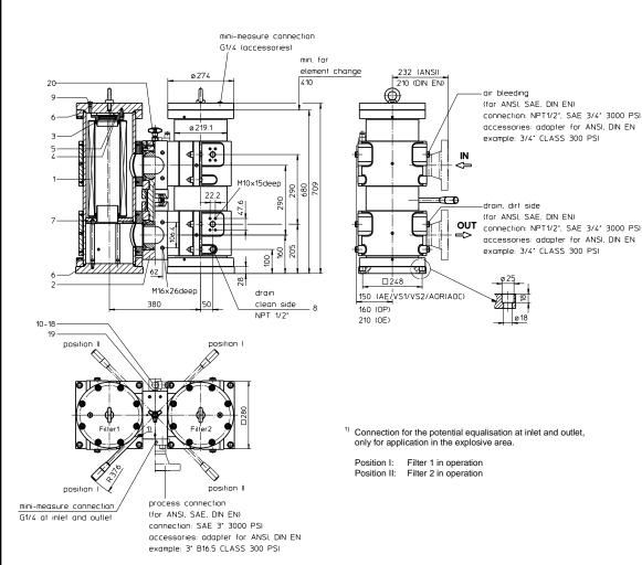
STAINLESS STEEL-PRESSURE FILTER, change-over Series EDA 1004 NPS 3" CLASS 300 PSI
