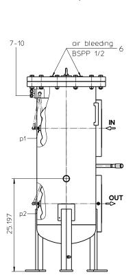
p1/p2 = mini-mesuring connection BSPP 1/4
