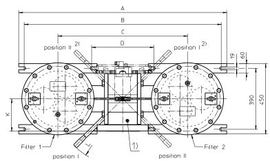
1) Connection for the potential equalization, only for application in the explosive area.
