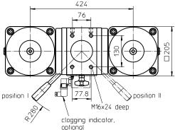
Position I: Left filter-side in operation Position II: Right filter-side in operation only for application in the explosive area.
