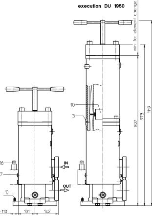
1) Connection for the potential equalization, only for application in the explosive area.
