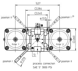
Position I: Filter 1 in operation Position II: Filter 2 in operation
