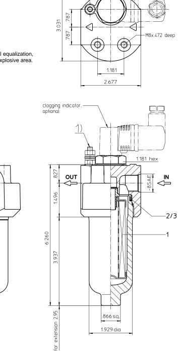
1) Connection for the potential equalization, only for application in the explosive area.
