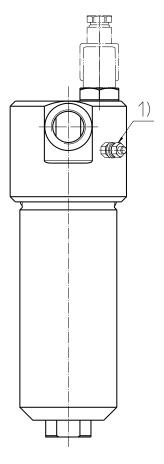
1) onnection for the potential equalization, only for application in the explosive area.
