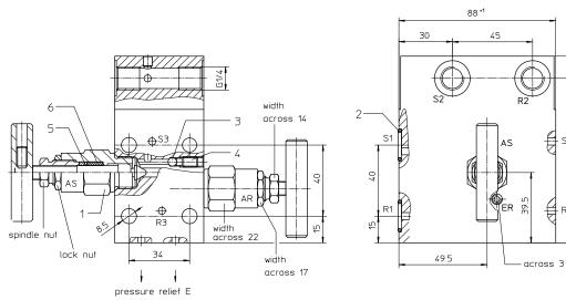
connection S3 and R3 only for intermediate plate construction
