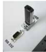
The CCS4 contamination control system is equipped with RS-232 and USB interfaces, and a number of accessories.
