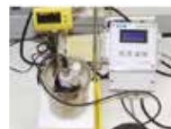
Water saturation determination with WSTM 01 set
