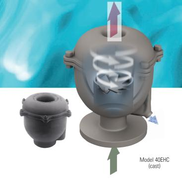
Eaton Type 40 Exhaust Heads are designed to separate entrained water and oil from exhaust air, gas, or steam prior to being discharged directly into the atmosphere. They remove more than 99% of liquids and solids over 10 microns in size from the discharged flow, reducing maintenance costs on roofs and surrounding objects.
