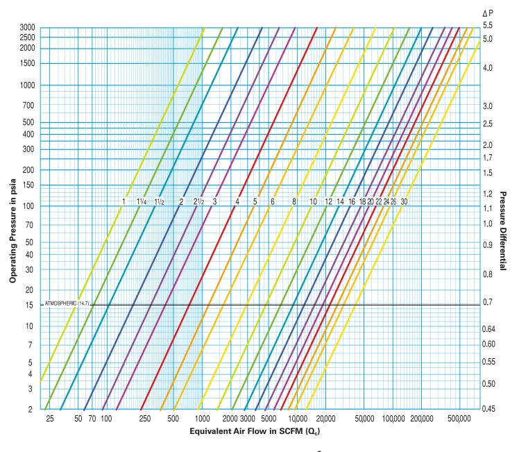
Application's Equivalent Air Flow SCFM (Q<sub>c</sub>) Separator's Maximum Rated Air Flow SCFM x Rated Pressure Drop Actual Pressure Drop = (obtain from scale at the right side of this chart)
