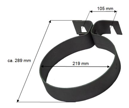
Set of wall mounting brackets (pair) consisting of clamp, each with a hex bolt and hex nut (M10). The clamp is designed for bag filter housings SIDELINE (SBF) and TOPLINE (TBF) sizes 01 and 02 and allows wall mounting.
